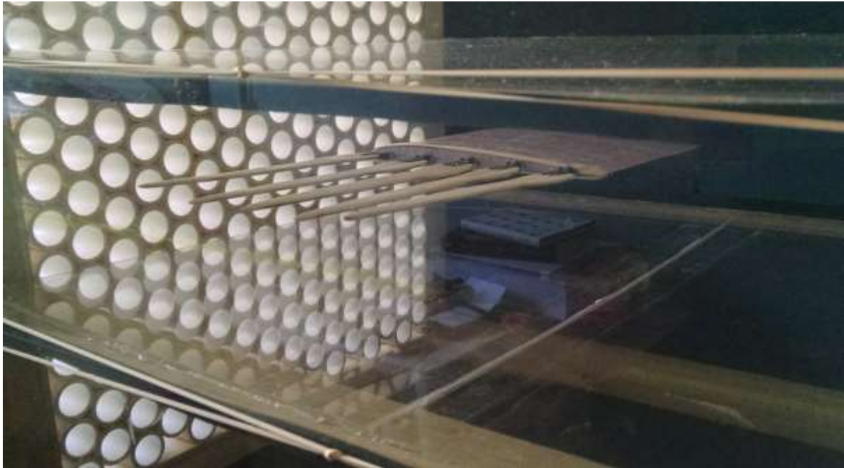
Figure 1: Multi-configurable Wing with Extensions Positioned in the Wind Tunnel
